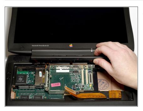
Lift the clutch cover off by rotating it up and then toward you.
