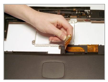
Turn the upper case over and pull the PMU connector cable up from the upper case.
