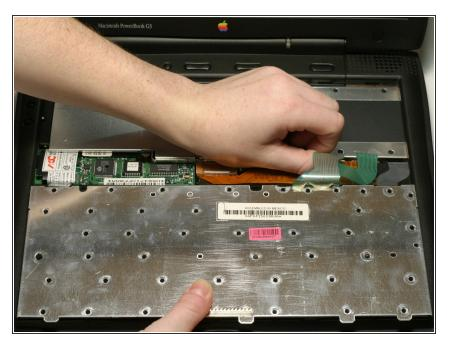
Disconnect the two keyboard connectors by disengaging the clamps and pulling the ribbons directly upward.
