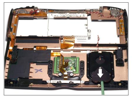
Use a spudger or the tips of your fingers to pry up the PRAM battery and free it from its housing.
