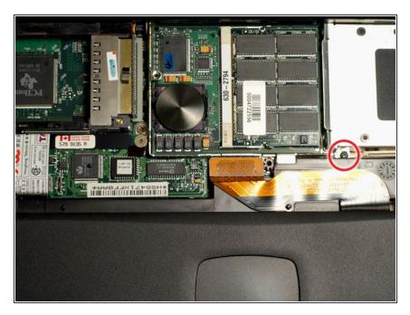
Unscrew, but do not remove, the single Phillips screw from the hard drive bracket.
