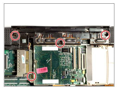
Remove the four T8 Torx screws from the upper case.
