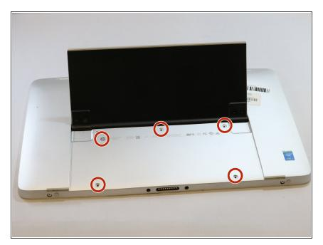
Remove five 4mm Phillips #0 screws securing the lower case to the HP Envy x2 13-j002dx.
