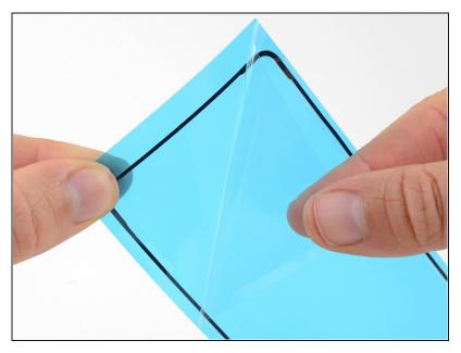
Peel the clear backing off of the replacement adhesive.
