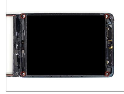
• Remove the four 3.9 mm Phillips #000 screws securing the LCD to the rear case.
