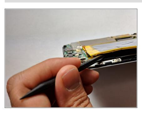
Carefully remove the battery by sliding a plastic spudger under the battery. Use an adhesive remover if available under the battery to make it easier for the battery to come off. To reassemble your device, follow these instructions in reverse order.
