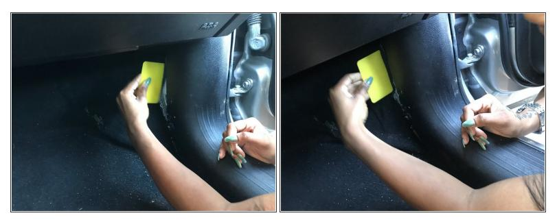
• Use a plastic squeegee to tuck the corner of the carpet into the paneling of the floorboard.
