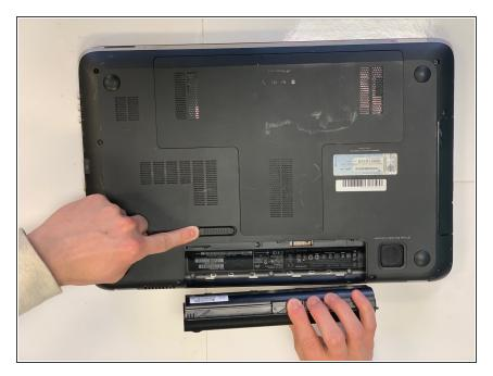
Firmly grasp the battery and remove it from the device.
