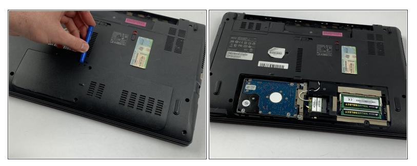
Use a spudger or plastic opening tool to lift the panel up. Then remove the panel entirely with your hands.
