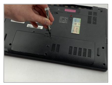
• Unscrew the two 8.6 mm screws using a Phillips #0 screwdriver.
