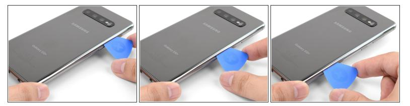
Slide the opening pick along the edge of the phone, slicing through the adhesive.
