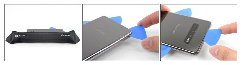
• Continue heating and slicing around the remaining edges of the phone.
