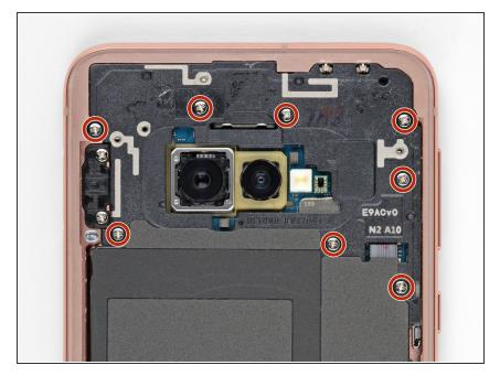
Remove the eight 3.9 mm Phillips screws securing the upper midframe to the phone.
