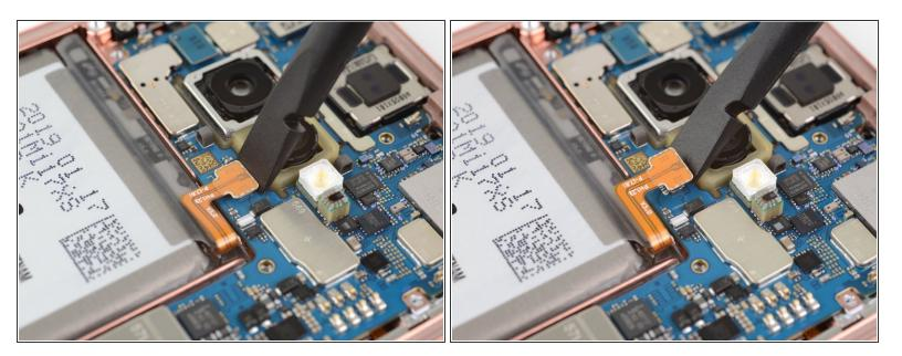
Use the flat end of a spudger to pry the battery connector straight up from its socket and disconnect it.
