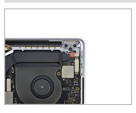
Use a T3 Torx driver to remove the 1.3 mm screw securing the cover bracket for the Touch Bar digitizer connector.
