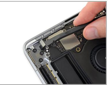
Disconnect the Touch Bar digitizer cable by prying it straight up from the logic board.
