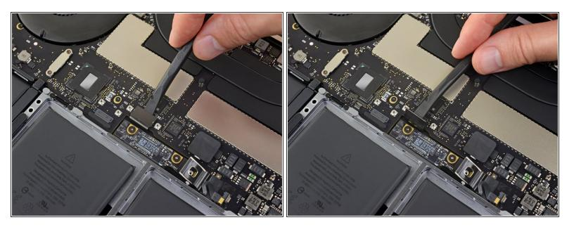
Use your spudger to disconnect the keyboard by prying its connector straight up from the logic board.
