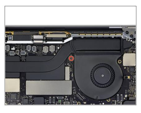
Use a T5 Torx driver to remove the single 2.9 mm screw securing the antenna cable bundle.
