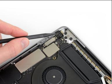
Disconnect the headphone jack cable by prying its connector straight up from the logic board.
