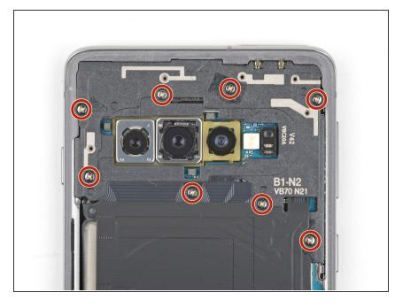
Remove the eight 4 mm Phillips screws securing the top midframe to the phone.
