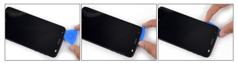
Insert an opening pick as deep as possible under the top left corner of the screen assembly to slice through the left patch of adhesive.
