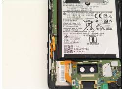
• Using the spudger, lift up the bar on the ZIF connector that joins the ribbon cable to the control buttons.
