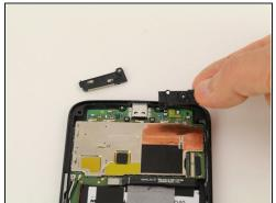
Unscrew four 1.8mm T4 screws from the speakers and remove from the motherboard.
