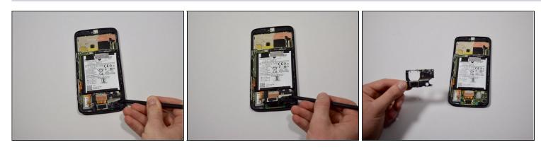
Use the nylon spudger to lift and remove the speaker from the phone chassis.
