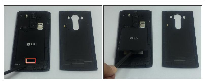
There's an impression next to the battery for the user to use their finger to pry the battery out; pry the battery out using your finger or the flat end of the spudger.
