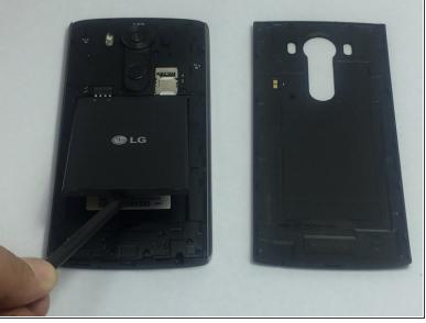
There's an impression next to the battery for the user to use their finger to pry the battery out; pry
