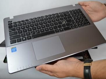
With the data cables removed and the keyboard module fully disconnected, the keyboard module should come free from the laptop.
