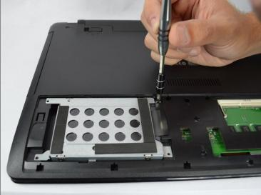
Remove the three 5mm screws holding down the hard drive and the five 5mm screws holding down the casing using a Phillips #00 bit.
