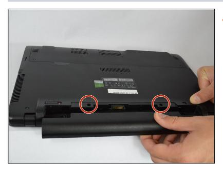
After detaching the battery, remove the two 5mm screws holding down the casing using a Phillips #00 screwdriver.
