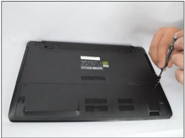
Loosen the four 12mm screws on the bottom and top panel of your device using a Phillips #0 screwdriver.
