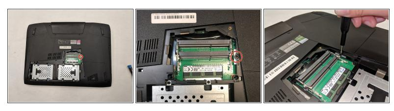
• Use a Phillips 1 Screwdriver to remove the 5 mm screw that is located underneath the back panel.
