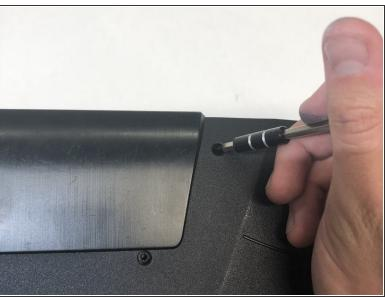
Use a Phillips 1 Screwdriver to remove the top four 8.5 mm screws.
