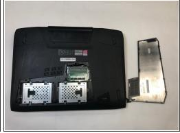
Use the standard spudger to remove the back center panel.
