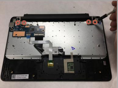
To free the hinge, remove the 4 mount screws with a Phillips #0 screwdriver.
