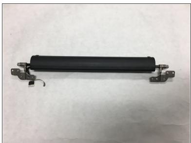
Remove the disconnected hinge from the keyboard.
