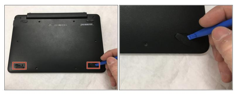
Turn over the keyboard and use the plastic opening tool to remove the two adhesive backed rubber pads furthest from the hinge.
