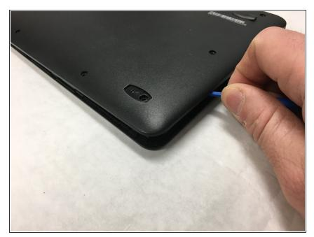
Use the plastic opening tool to separate the front and back halves of the keyboard.
