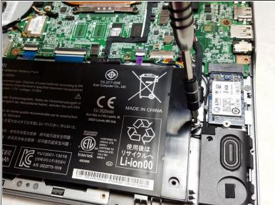
Remove the two 3mm screws using the Phillips #0 screwdriver.
