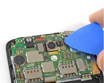
• Use the tip of an opening pick to pry up and open the black lever of the ZIF connector located at the top of the motherboard next to the rear camera.
