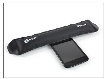
Prepare an iOpener and apply it to the upper half of the display for at least two minutes to loosen the adhesive beneath the vibration motor and the rear facing camera.
