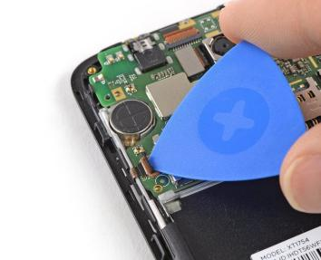
• Use the tip of an opening pick to pry up and open the black lever of the ZIF connector located on the bottom left of the motherboard.
