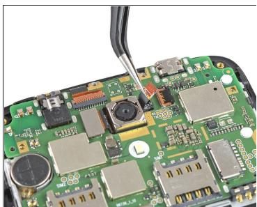
• Use a pair of tweezers to pull the digitizer flex cable out of the ZIF connector.
