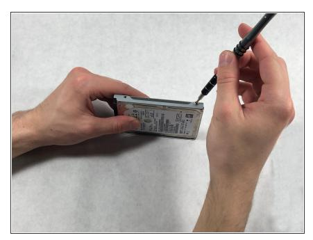
Using a Phillips #0 screwdriver, remove the four Phillips M3.0×3.5 screws (two on either side of the hard drive).
