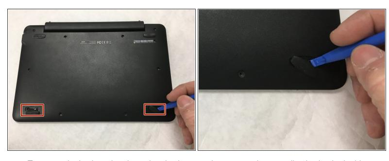
Turn over the keyboard and use the plastic pry tool to remove the two adhesive backed rubber pads furthest from the hinge.
