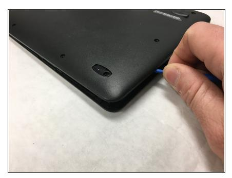
Use the plastic opening tool to separate the front and back halves of the keyboard.
