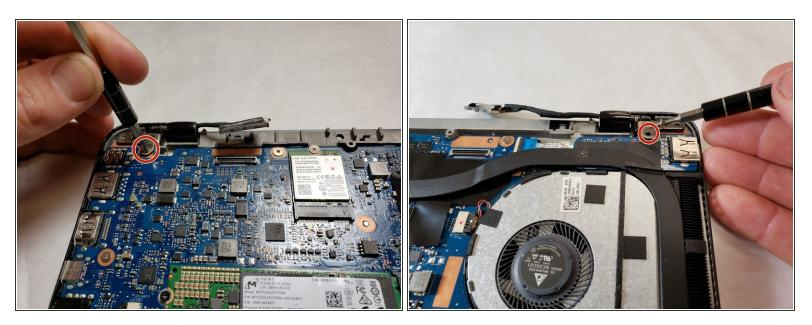
Remove two 6 mm screws using a Phillips #0 Screwdriver.
