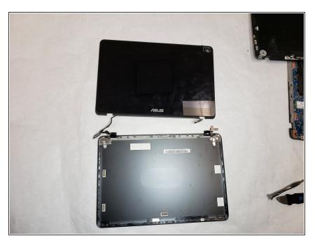
• Remove the display from the device.
