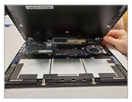
• Remove the back plate to access internal components.
