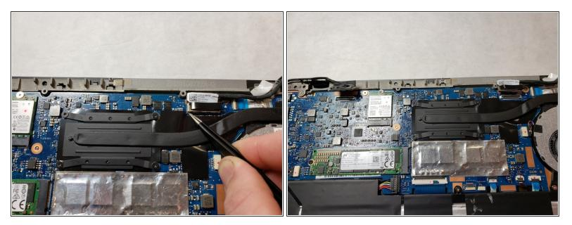
• Use a pair of tweezers to disconnect the two black rectangle connections.
