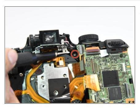
Use the Phillips screwdriver to remove the single 6 mm screw.
