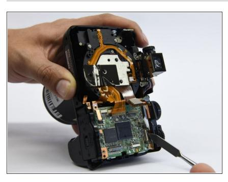
• Use the metal spudger to open the latch to remove the ribbon.
