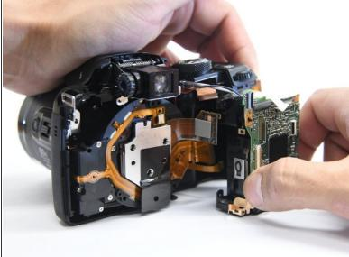
• Gently lift the button assembly. Slide the motherboard out from the shell.
