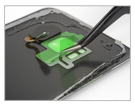
Peel the green backing away from the adhesive strip. Make sure the adhesive does not come off of the glass with the backing.
