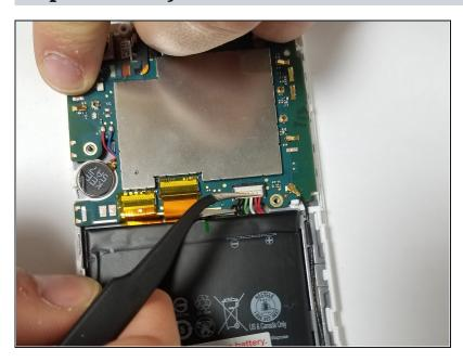
By using the angled tweezers, you have to be careful when you try to remove the battery connection by start pulling the wires.
