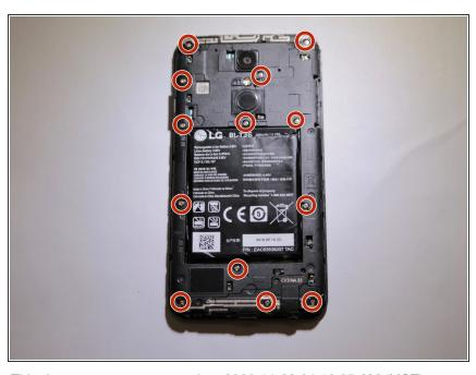
Remove the thirteen 3.4 mm Phillips #00 screws securing the midframe to the display assembly.
