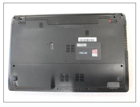
Press and slide the two battery retention clips on either side of the battery towards the unlock position.
