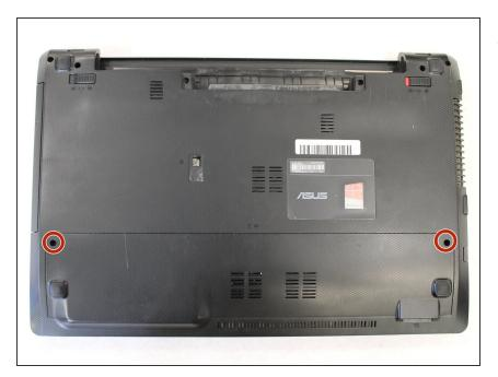
• Remove the two 8.5mm screws using a PH0 screwdriver.
