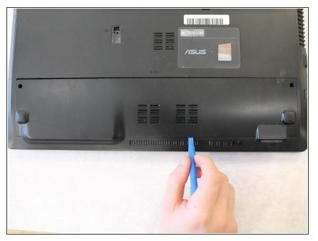
• Using the iFixit opening tool, gently pry the plastic cover away from its original position.
