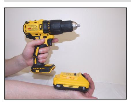
Pull the battery in a horizontal direction away from the drill.
