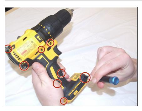
Remove the eight 16 mm screws by using a Torx Security #15 screwdriver.
