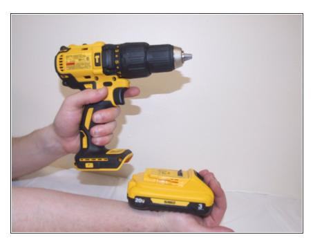
Remove the battery from drill by sliding the battery outwards away from the drill.
