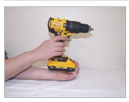
Compress the button on front side of the battery and move the drill and battery away from each other.
