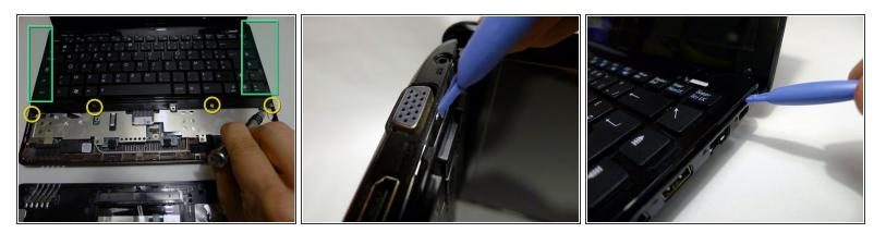
Make sure that the two upper screws inside the RAM compartment are removed before to continue. (Refer to Step 5).
