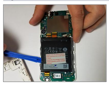
Using the plastic opening tool to separate the battery and remove it.
