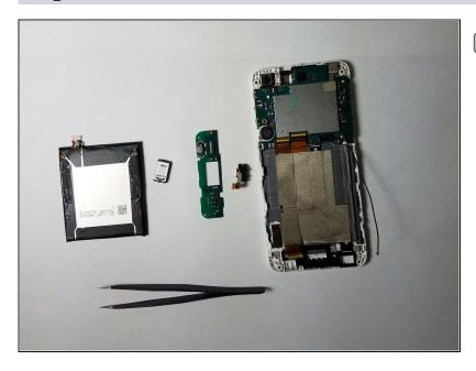
The new board will not go in as easily as the old one came out. Just be patient and squeeze the edges to clip it into place.
