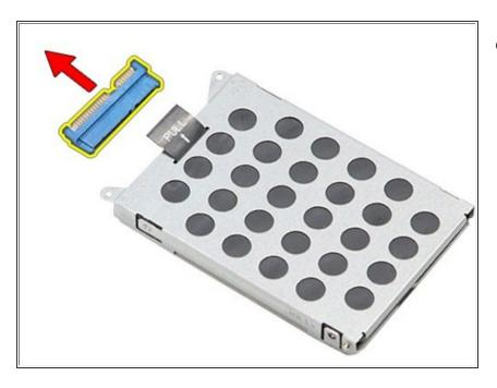
Remove the hard-drive adapter from the hard-drive assembly.
