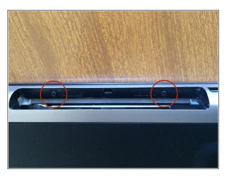
With the laptop closed, lay it upside down on the bench and remove 2 screws from the CD/DVD bay opening.
