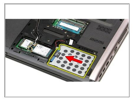
Slide the hard-drive assembly towards the center of the computer.
