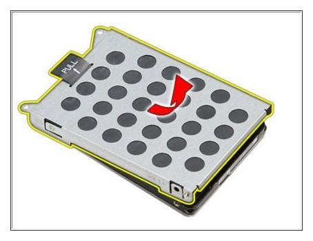
Lift the hard-drive bracket up and away from the hard drive.
