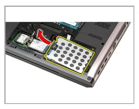
Lift the hard-drive assembly up and away from the computer.
