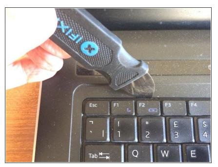
• There are 4 tabs along the top of the keyboard and two along each side which need to be released. The
