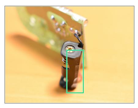
Cut down the lower back edge of the battery holder
