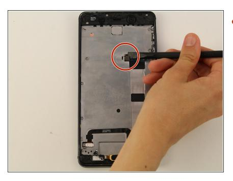
Disconnect the battery connector with a spudger.
