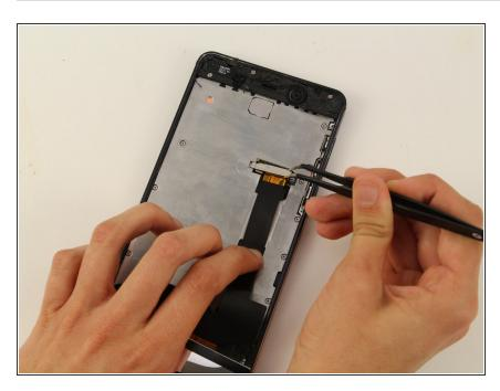
Remove the metal bracket with a tweezer.
