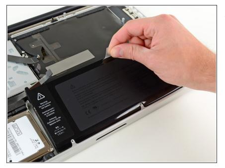
Use the attached plastic pull tab to remove the battery from the upper case.
