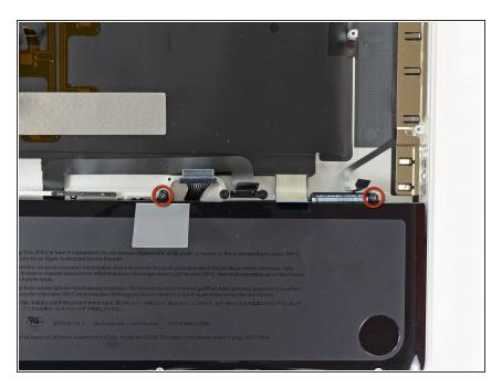
Remove the two 7.5 mm (7.2 mm) Tri-point screws securing the battery to the upper case.
