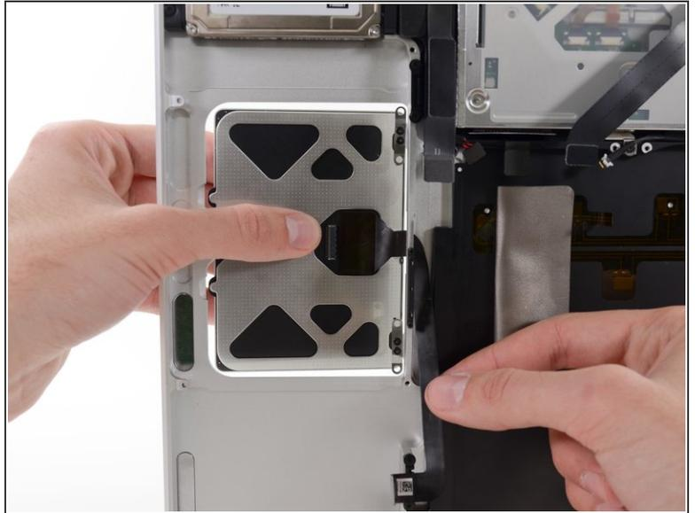
**i** While keeping a hold on the trackpad ribbon cable with one hand to keep it from tearing or creasing, ease the trackpad out of the upper case.
