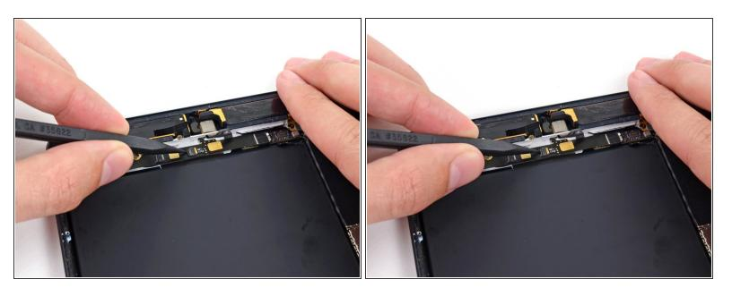
Use the tip of a spudger to lift the tab on the microphone data cable ZIF connector.
