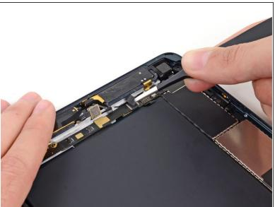
Peel up and remove the small piece of tape covering the headphone jack cable connector.
