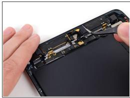
Use tweezers to peel and remove the long thin black tape covering the top of the headphone jack cable.
