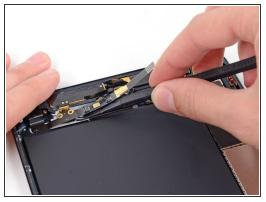
Slide the flat end of a spudger beneath the length of the headphone jack cable, separating the adhesive securing the cable to the rear case.
