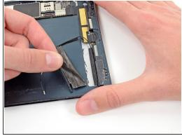
Peel back and remove the wide tape from the iPad.
