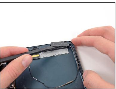
Use the flat end of a spudger to loosen the foam adhesive securing the lower left antenna to the left speaker.
