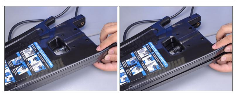
Separate the bottom edge of the handle slightly until the spring-loaded plunger pops out of its socket.
