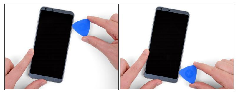
Slide your opening pick down the final long edge of the phone to separate the last of the adhesive holding the screen in place.
