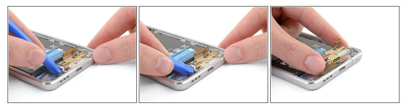
Use the flat end of an opening tool to pry up the USB-C / mic assembly and remove it from the phone.
