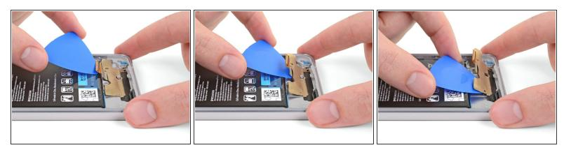
• Slide an opening pick under the display cable to separate the adhesive holding it in place.
