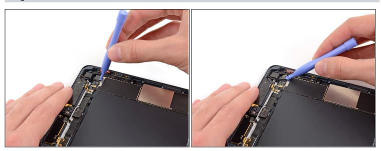
• Pry the rear-facing camera connector up out of its socket in the logic board.
