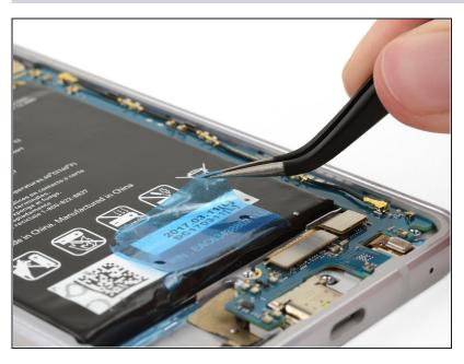
Use <u>tweezers</u> to lift up the blue pull tab at the bottom of the battery.
