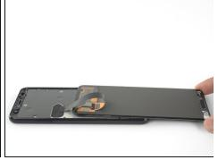
With all of the adhesives cut, flip the attached screen glass side down and rest it on top of the phone. The screen flex cable should be loosely arched.
