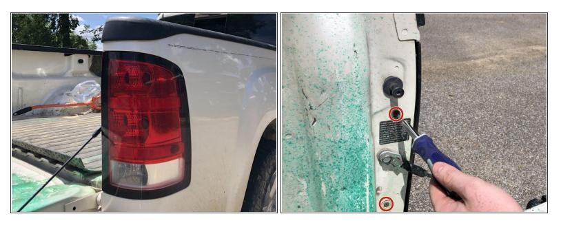
Using the Philips screwdriver, remove the two 4.8x16mm screws securing the housing.
