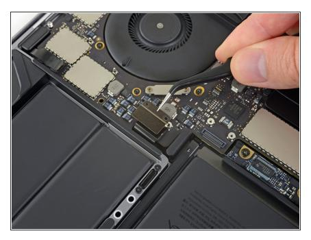
Remove the keyboard connector bracket.
