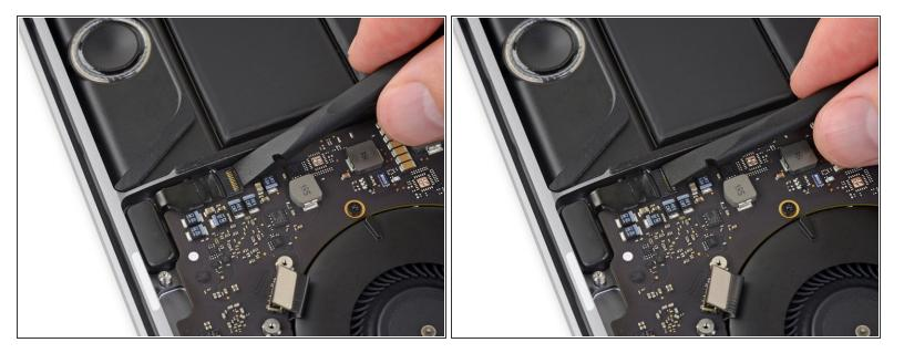
Flip open the locking flap for the right-side tweeter ZIF connector by prying it straight up from the logic board.
