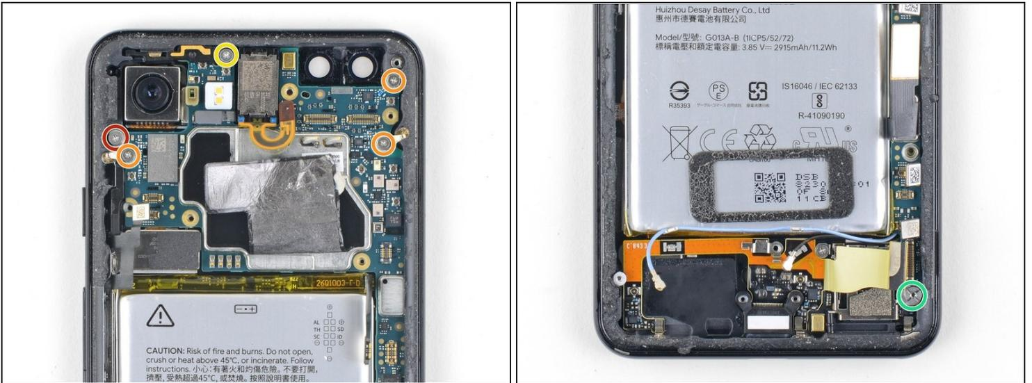
**i** Some of these screws hold very small grounding clips in place. *Be careful not to lose these clips* as you remove the screws.
