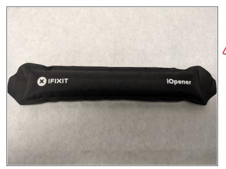
• Heat up the iOpener in the microwave for 30 seconds.
