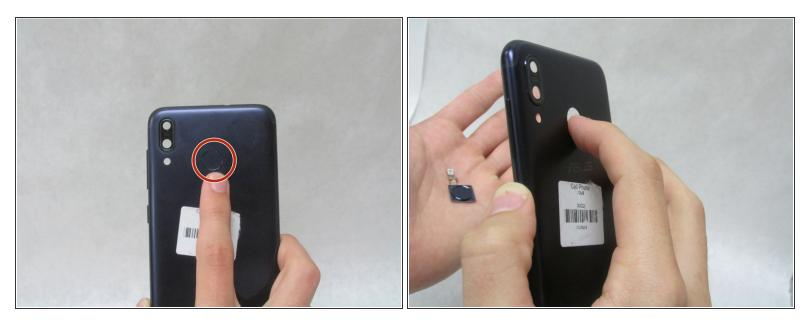
• On the back shell of the phone, push with pressure on the touch sensor until it pops out.
